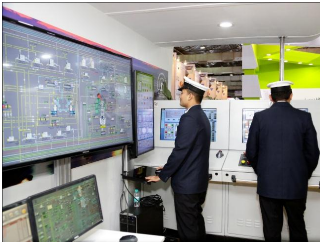
ARI Engine Room Simulator with interactive 3D Engine Room
